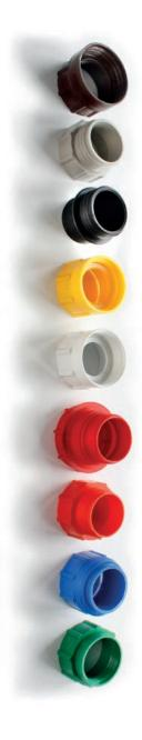
Thread adapters for equalization of different threads at canisters, drums, containers, etc. when fixing f.e. hand pumps. In principle the JESSBERGER hand pumps can be screwed due to their already existing drum adapters (2" BSP male thread) easily into the threads of steel drums like S 60 or S 200.
